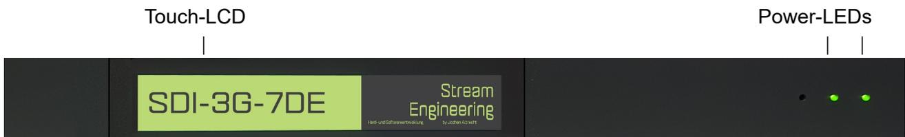
The LC-Display shows the type of 3G-SDI Inserter. When pressing the touch-display, the actual state, then detailed device information and network settings will be shown.
